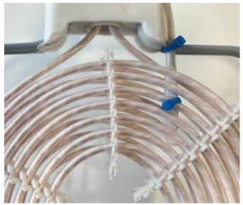
The probe is mounted along the non-heating part of the immersion heater (N cable) using PP (polypropylene) clamps. The sensitive part of the probe is inserted between the heating coils and held in place with 2 ETFE clamps.
